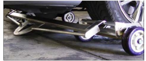
11.) ATTACH WINCH CABLE TOW HOOK TO FRONT OF TOW BAR AND TAKE UP THE SLACK IN WINCH CABLE. THIS WILL PREVENT THE VEHICLE FROM ROLLING BACK.
