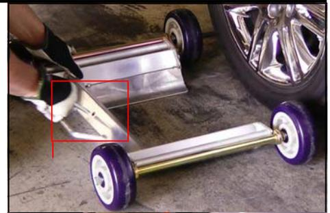
2.) SLIDE DOLLY APART UNTIL LEGS CAN BE PLACED FORE AND AFT OF VEHICLE'S TIRE.
