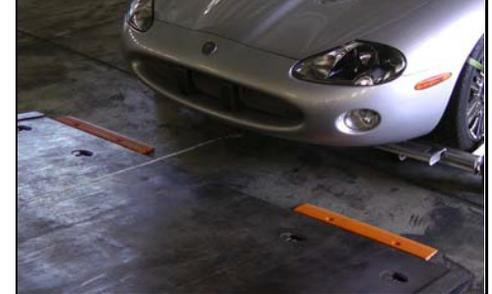
14.) VEHICLE IS NOW READY FOR WINCHING UP CARRIER BED. ONCE LOADED, SECURE VEHICLE TO BED AS USUAL, LEAVING THE VEHICLE ON THE DOLLIES.
