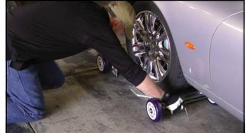
4.) TIGHTEN DOLLY LEGS AGAINST VEHICLE'S TIRE THEN REPLACE LOCK PIN THROUGH HOLES IN TELESCOPIC ARM.
