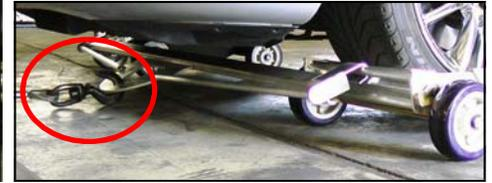
12.) WITH VEHICLE SECURED TO CARRIER'S WINCH CABLE, PUT FOOT ON BRAKE AND PLACE VEHICLE TRANSMISSION IN **NEUTRAL**. THEN RELEASE PARKING BRAKE. IF THERE IS NO ACCESS TO VEHICLE, A SECOND SET OF MINI DOLLIES WILL BE NECESSARY TO CARRY THE TRAILING AXLE OF THE VEHICLE.
