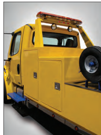
Tunnel Box with 6" Step Down
