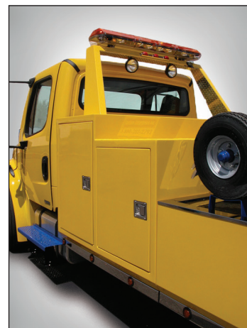
Tunnel Box with 6" Step Down
